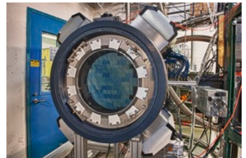
570 megapixel DES camera (DECam), holds 74 CCDs ( www.darkenergysurvey.org )
